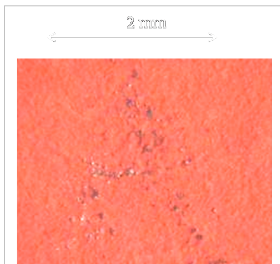
Figure 3. Track left by a Pb stylus on paper prepared using a mixture of cinnabar (HgS) and lead-white ((2PbCO 3 Pb(OH) 2 )
