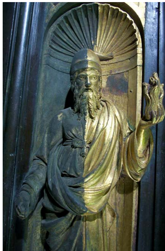
Figure 5. A frieze of the Porta del Paradiso by Lorenzo Ghiberti during the laser cleaning intervention. The gold film behind the dark deposit of soot, carbon particles and salts is perfectly preserved.
