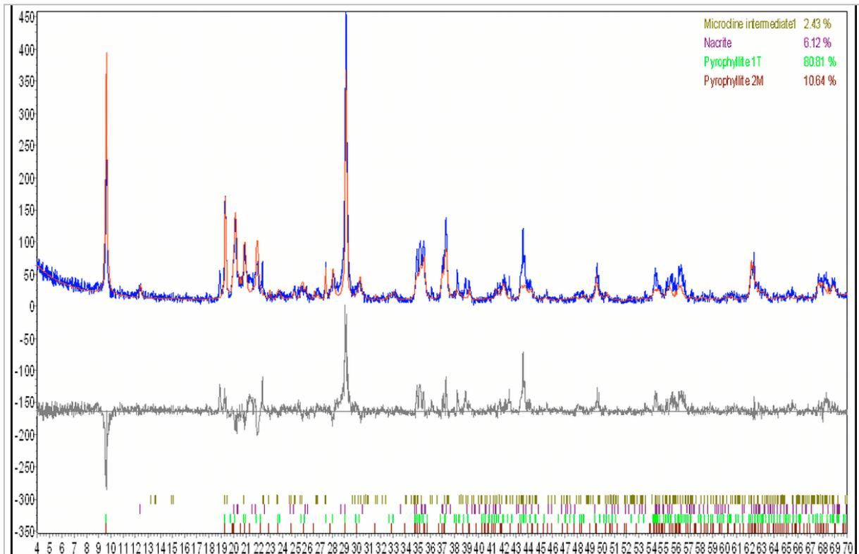
**Fig. 18.** - Rietveld refined diffraction pattern of commercial pyrophyllite
