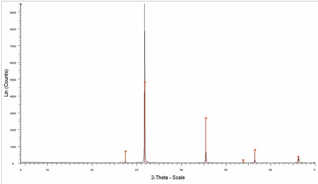
**Fig. 10.** - Diffraction pattern of cubic rocksalt
