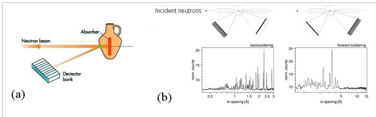
**Figure 2.** (a) TOF-ND schematic; (b) patterns collected with detectors at different angles provide different d-spacing ranges with different d-resolutions
