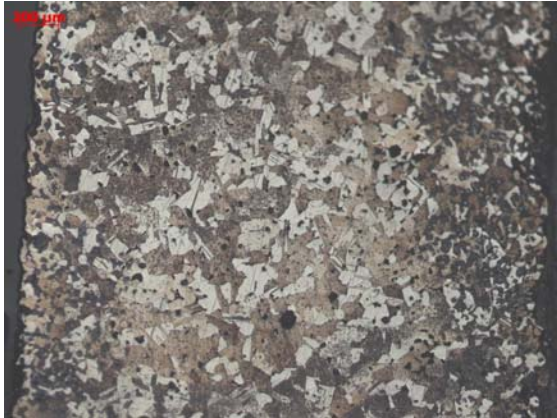
Fig. 6.: The microstructure of the cauldron-fragment. Recrystallized grains and intensive corrosion revealed by the optical micrograph. The corrosion can be discovered mainly at the grain boundaries. Zeiss Axio Scope.A1. Magnification.: 50x. Etching.: \text{FeCl}_3 , Bright Field
