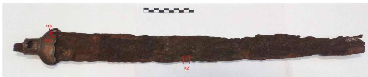
Fig. 1.: The places of sampling on the sword (sample K1A, K1B and K2)
