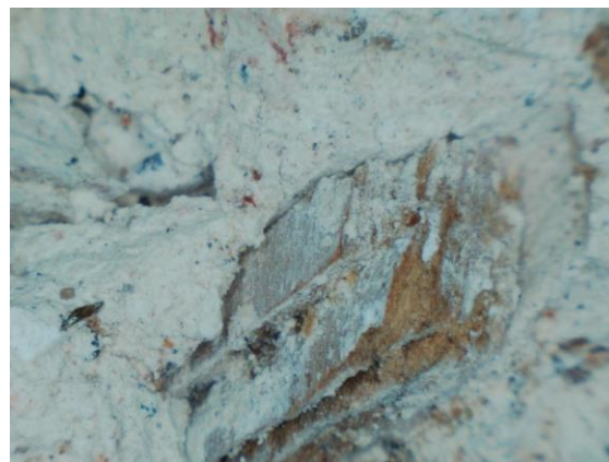
Fig. 2.: Fragment of wood inside the 12 th century intonaco . The fragment is not prepared to show the wood fragment as found. The plaster is very white, with only few wood fragments and no sand. Magnification 50x (Photo by authors)
