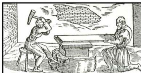
16 th century goldbeaters at work on a duplex plate of gold and silver [3].
