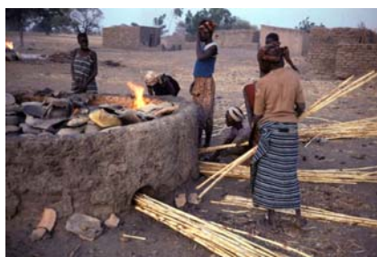
The round enclosed fire kiln
