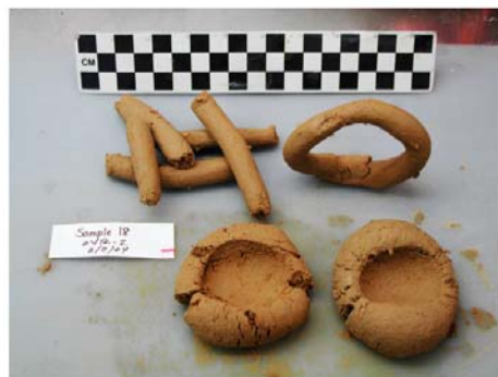
Figure 4.11. A lean sample (FBR015). Note the broken coil (upper left), sagging loop (upper right), and deeply cracked ball (bottom).
