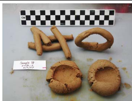
Figure 4.11. A lean sample (FBR016). Note the broken coil (upper left), sagging loop (upper right), and deeply cracked ball (bottom).
