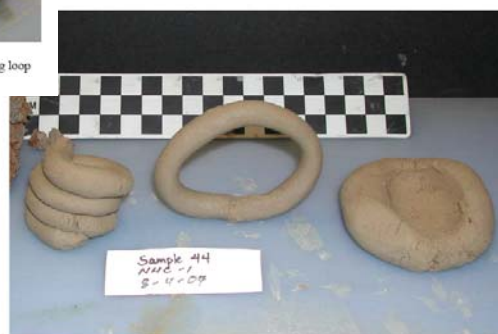
Figure 4.12. A good sample (FBR040). The coils and ball did not crack, and the loop retained its shape.
