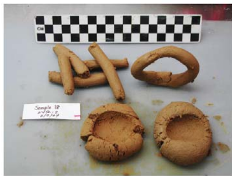
Figure 4.11. A lean sample (FBR015). Note the broken coil (upper left), sagging loop (upper right), and deeply cracked ball (bottom).
