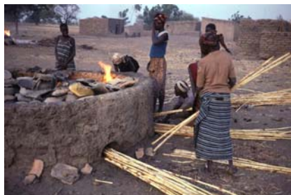
The round enclosed fire kiln
