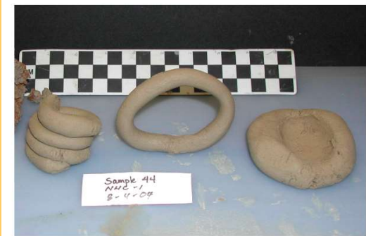
Figure 4.12. A good sample (FBR040). The coils and ball did not crack, and the loop retained its shape.
