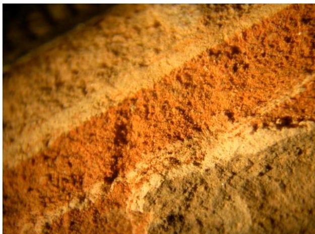
Fig. 4a Layers of a daub fragment (on the scale the distance between two signs is 1 mm)
