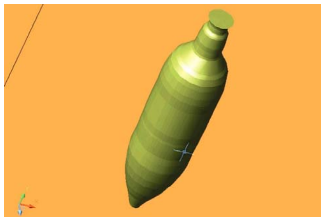
Fig. 6 End product: 3-D solid used for vessel capacity calculation
