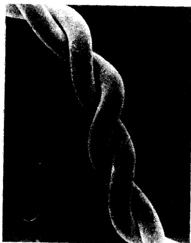
Fig. 4,5,6: Scanning electron micrograph of three metal embroidery threads of a 17th century coat /Esterházy Collection/
